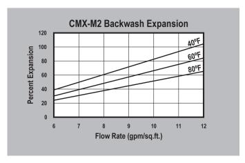
**CMX-M2 BACKWASH** — The graph above shows the expansion characteristics as a function of flow rate at various temperatures.
