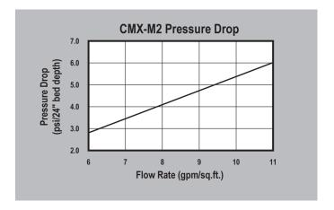
**CMX-M2 PRESSURE DROP** — The graph above shows the expected pressure loss per 24 inches of bed depth as a function of flow rate.
