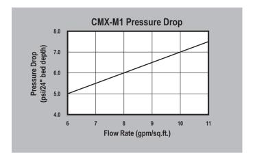
**CMX-M1 PRESSURE DROP** — The graph above shows the expected pressure loss per 24 inches of bed depth as a function of flow rate.
