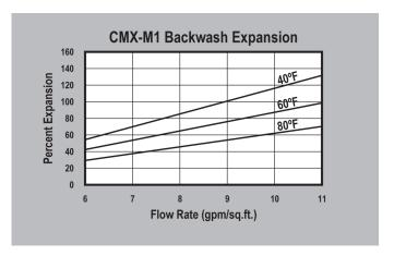
**CMX-M1 BACKWASH** — The graph above shows the expansion characteristics as a function of flow rate at various temperatures.
