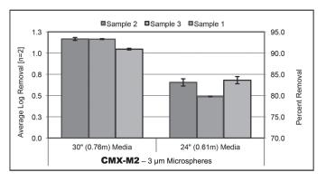
3 to 5 micron microsphere log removal Average removal 30 inches of media 90% Average removal 24 inches of media 79%
