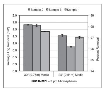
3 to 5 micron microsphere log removal Average removal 30 inches of media 97.1% Average removal 24 inches of media 94.8%
